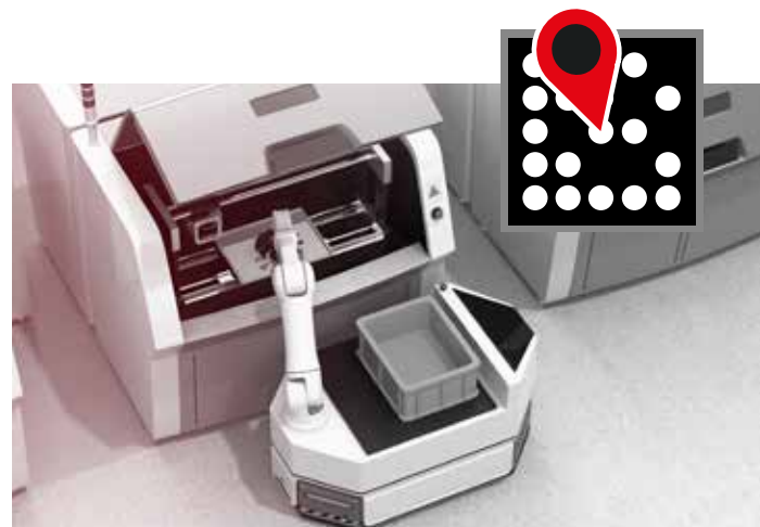
Target Mark technology enables easy identification and precise referencing of your mobile work stations.
