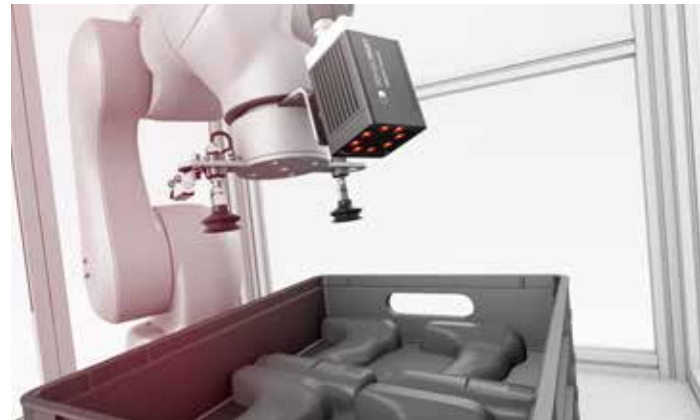
The position of components supplied in a tray can vary so strongly that robot guidance is necessary.
